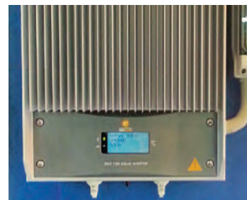
Inverter for typical grid-tied system used in some Schoolgen Schools
