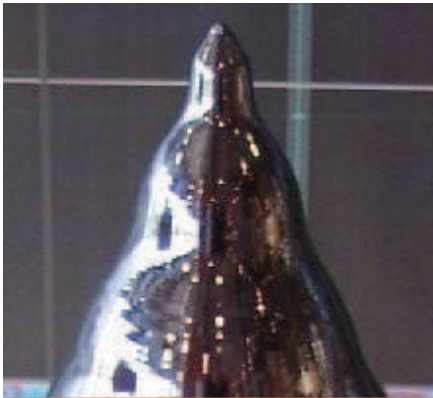
Boule of monocrystalline silicon grown from a silicon seed crystal
