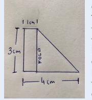
Cut out the 3 fins. Tape these on to the rocket with the pencil still inside so that you can press the tape hard. You need to tape on both sides of the fins.
