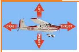
One of the four forces of flight is thrust. This is the force that propels the plane forward.
